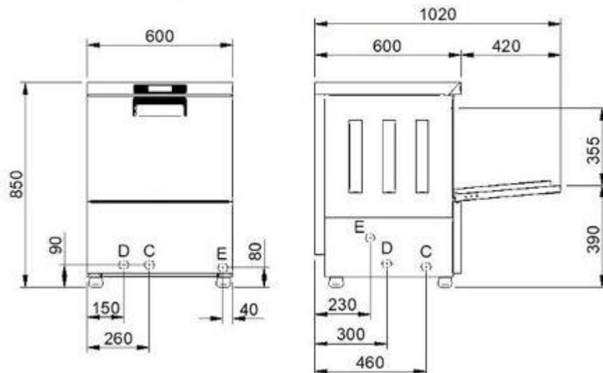
**D** = SCARICO 1 1/2", VIDANGE 1 1/2", DRAIN 1 1/2"; ABFLUSS 1 1/2"; DESAGÜE 1 1/2"; СЛИВ 1 1/2"
